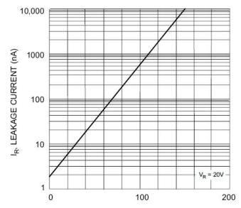
$\label{eq:tj} \textbf{T}_{j}, \, \text{JUNCTION TEMPERATURE (°C)} \\ \text{Fig. 2 Leakage Current vs Junction Temperature}$
